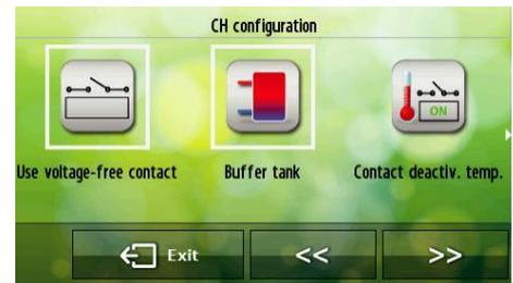
The regulator has a voltage-free output which opens (or closes) contact when CH temperature reaches the value preset by the user. The setting range for this parameter is 30÷75°C.
