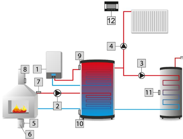
The EU-392 zPID temperature regulator is designed for wall mounting. It is powered from the main module via the RS connector.
