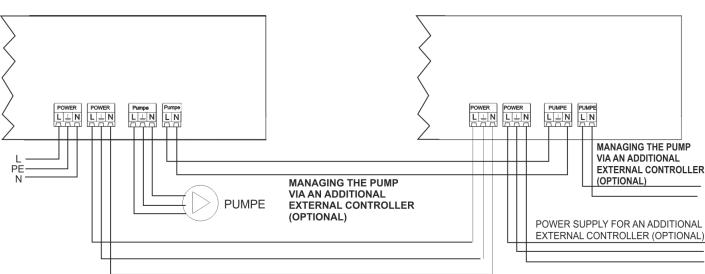
POWER SUPPLY FOR AN ADDITIONAL EXTERNAL CONTROLLER (OPTIONAL)
