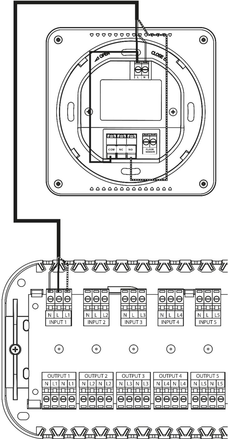
➤ Connection of actuators and room regulators - batteries
